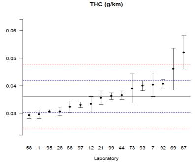
Figure 03 – Scatter plot of the results for THC determination
