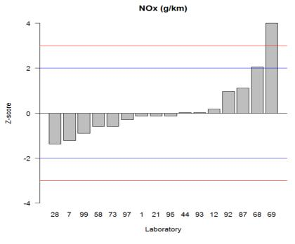
Figure 14 - z-score graph of for NO<sub>x</sub> measurement
